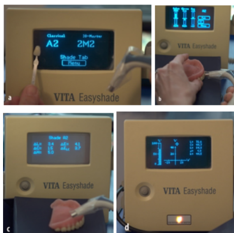
Fig. 1. Vita Easyshade spectrophotometer was used to perform measurements: a – A2 shade tab from the Vitapan Classical shade guide was verified prior to any measurement. b-Positive control (PC) was compared to A2 shade using the option Restoration. The differences of Value, Chroma and Hue are represented and Fair is the overall color accuracy. c- The screen shows the positioning of the tooth's color measured with respect to the color space coordinates for the A2 shade. ΔE is the color difference calculated using CIE L*a*b* system and ΔE LC is calculated excluding H. d -Color coordinates in CIE L*a*b* system (L, a, b, C, H) for the measured specimen using the Tooth single option are displayed on the screen
